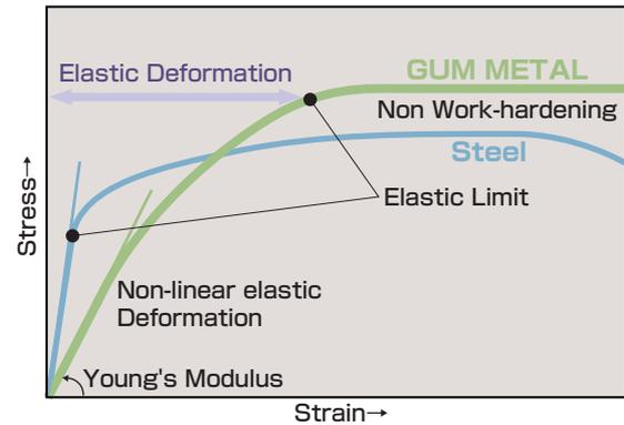
nature (Fig.2). Since the alloy does not show work-hardening at all under any kind of hard working, continuous deformation is possible to any desired level.
